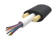
Fiber outdoor drop cable, LightScope® ZWP Self-Supporting All-Dielectric, Singlemode G.652.D and G.657.Al, 2 fiber Arid Core construction, Gel-filled, central loose tube, Feet jacket marking, Black jacket color
