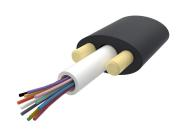
Fiber outdoor drop cable, LightScope® ZWP Self-Supporting All-Dielectric, Singlemode G.652.D and G.657.Al, 8 fiber Arid Core construction, Gel-filled, central loose tube, Feet jacket marking, Black jacket color
