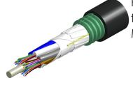
Fiber OSP cable, LightScope® ZWP Mini Single Jacket/Single Armor, 24 fiber, Gel-Filled, Stranded Loose Tube, Singlemode G.652.D and G.657.A1, Meters jacket marking, Black jacket color
