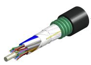
Fiber OSP cable, LightScope® ZWP Mini Single Jacket/Single Armor, 48 fiber, Gel-Filled, Stranded Loose Tube, Singlemode G.652.D and G.657.Al, Meter jacket marking, Black jacket color
