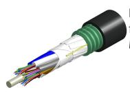
Fiber OSP cable, LightScope® ZWP Mini Single Jacket/Single Armor, 72 fiber, Gel-Filled, Stranded Loose Tube, Singlemode G.652.D and G.657.Al, Meters jacket marking, Black jacket color
