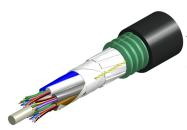
Fiber OSP cable, LightScope® ZWP Mini Single Jacket/Single Armor, 144 fiber, Gel-Filled, Stranded Loose Tube, Singlemode G.652.D and G.657.Al, Meters jacket marking, Black jacket color
