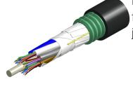
Fiber OSP cable, LightScope® ZWP Mini Single Jacket/Single Armor, 48 fiber, Gel-Filled, Stranded Loose Tube, Singlemode G.657.A2, Meters jacket marking, Black jacket color
