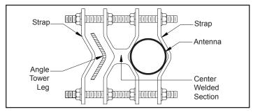
Figure 2. Mounting on Angle Tower Legs.
