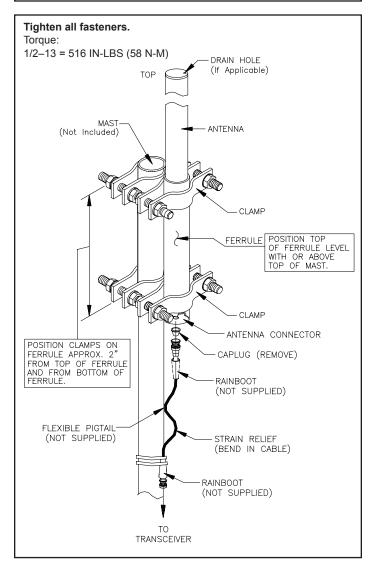
Figure 4. Upright Mounting of Antenna.
