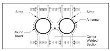
Figure 1. Mounting on Round Tower Legs.
