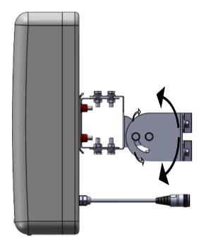
1. Loosen the fixing screws. (Do NOT unscrew them completely.)
