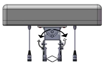
1. Loosen the fixing screws. (Do NOT unscrew them completely.)
