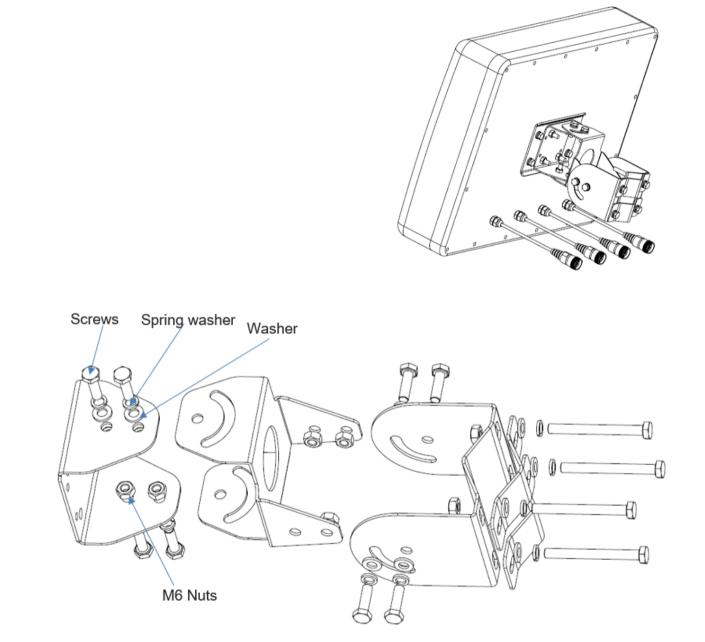
Fit these seven parts above together and fasten them with screws M6, nuts M6, spring washers, and washers.
