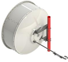
1.8 m | 6 ft ValuLine® High Performance Low Profile Antenna, single-polarized, 7.125–8.500 GHz, PDR84, white antenna, flexible woven polymer gray radome without flash, standard pack—one-piece reflector
