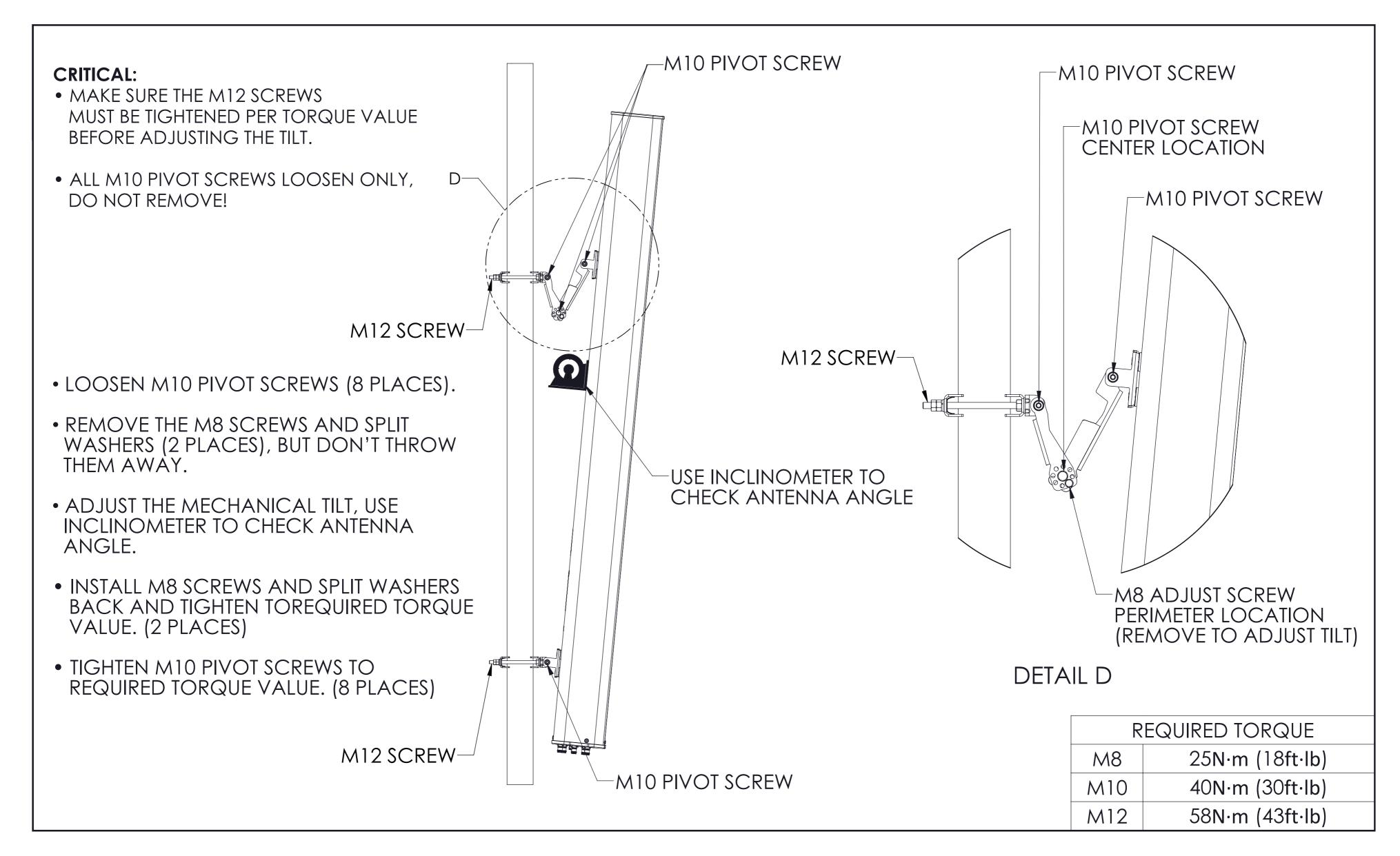
ADJUSTING ANTENNA TILT - 2 POINT MOUNT (NOT APPLICABLE FOR BSAMNT-F)
