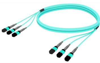
Ultra Low Loss (ULL) OM4 MPO8 QSFP (Pinned) to MPO8 QSFP (Pinned), Armored Fiber Trunk Cable Assembly, 24-Fiber, Plenum
