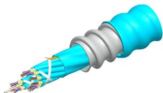
LazrSPEED® Plenum MPO Trunk Cable, interlocking aluminum armored with plenum jacket, 24 fiber with 12 fiber subunits
