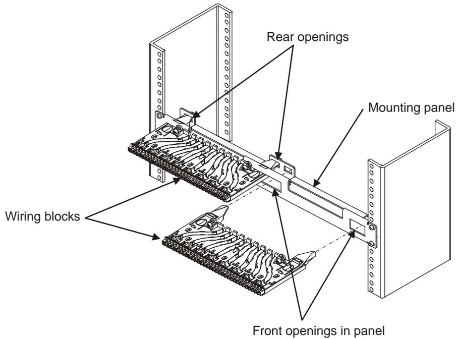
1. Insert wiring blocks into front and rear openings in mounting panel until an audible click is heard.
