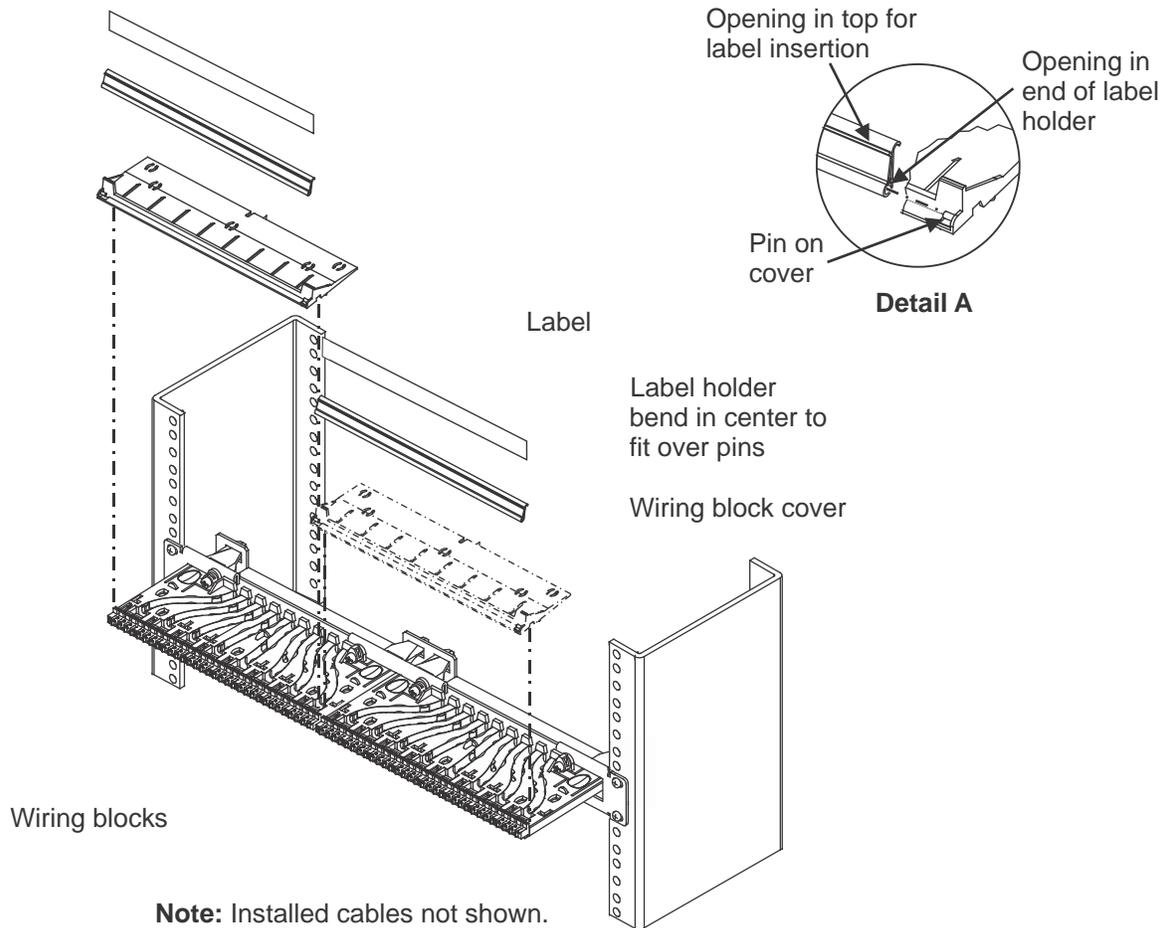
1. Position cover as shown above and push down onto wiring block until latches in cover engage in wiring block.
