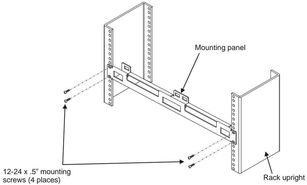
1. Orient mounting panel as shown above and install on rack using the four 12-24 x .5" screws provided.
