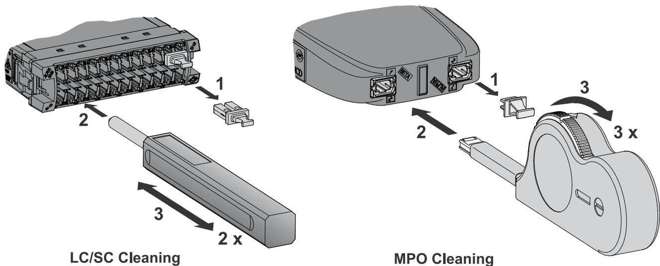
Clean each module port prior to installing a mating connector.
