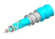
Fiber indoor cable, LazrSPEED® Riser/LSZH rated, MPO Trunk, interlocking aluminum armored, Multimode OM4, 96 fiber, Gel-free, Feet jacket marking, Aqua jacket color, B2ca flame rating
