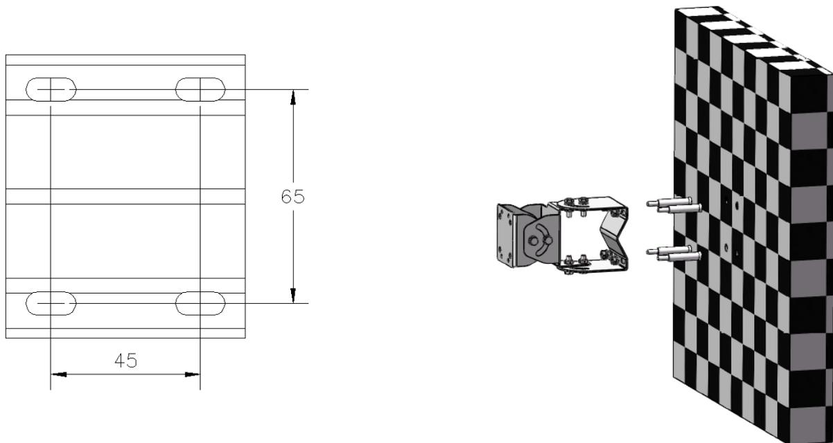
1. Use this pedestal piece as a drill jig to mark 4 holes onto the wall as shown in the drawing above.
