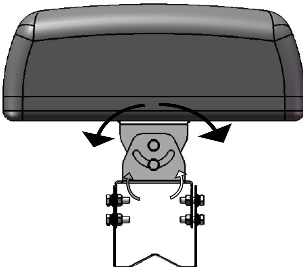
1. Loosen the fixing screw. (Do NOT unscrew it completely.)
