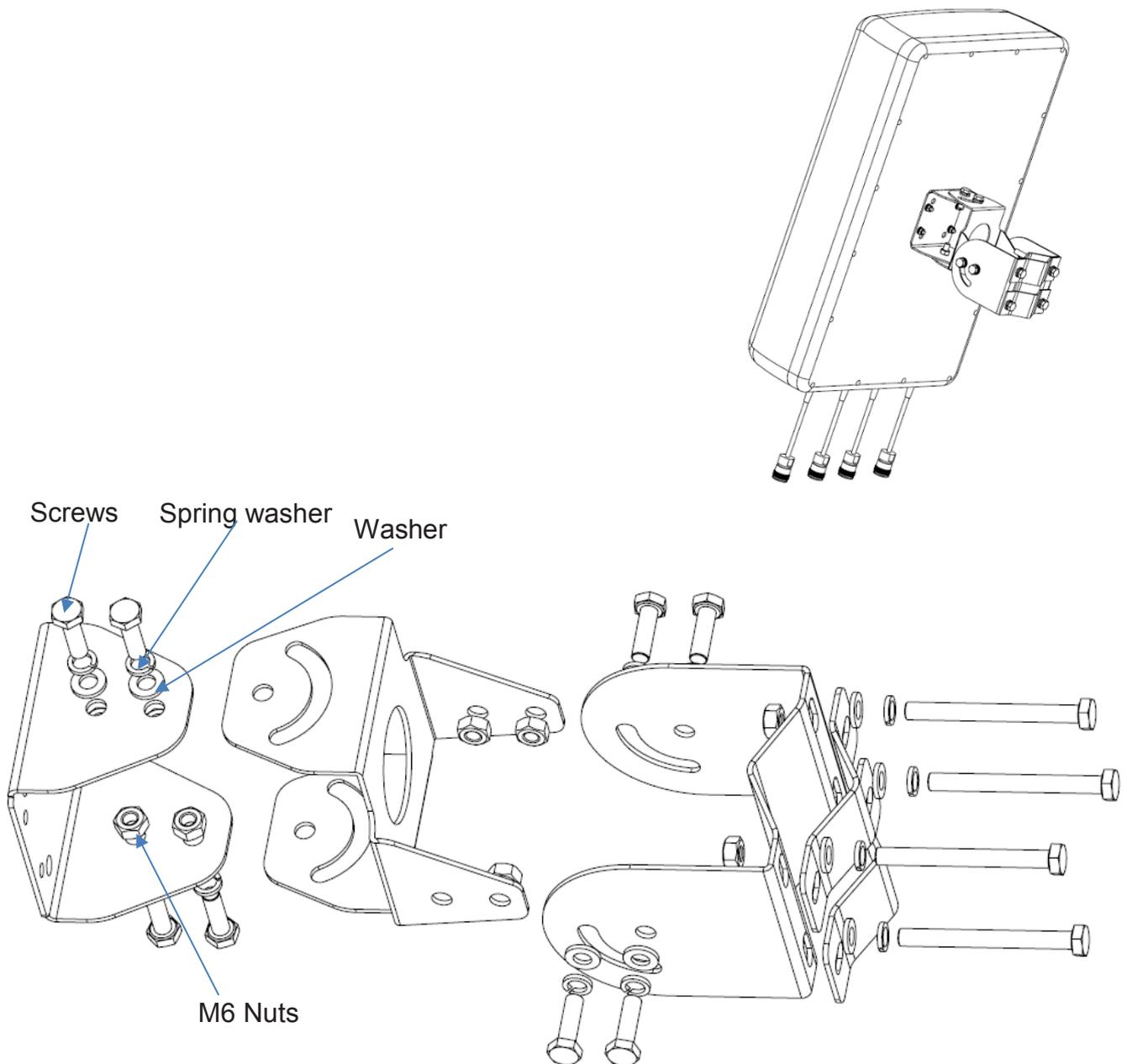
Fit these seven parts above together and fasten them with screws M6, nuts M6, spring washers, and washers.
