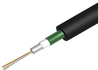
Fiber OSP cable, PE, Gel-filled Central Tube, CST, 12 fiber, Singlemode G.652.D and G.657.A1, Meters jacket marking, Black jacket color
