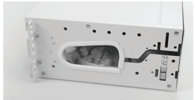
4.8 Install the edge protector on the entrance cable area side.
