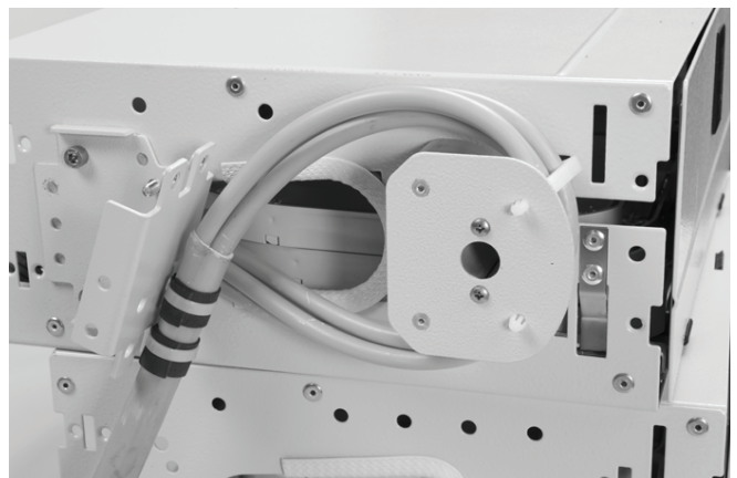
5.2.19 Install the edge protection at the bottom of the opening. Mount the drum on the side panel. Cut the strength member to 35 mm maximum. Attach the strength member and install as shown. Same installation and routing for break-out cable. Recommended to use GTU (see section 5.2).
