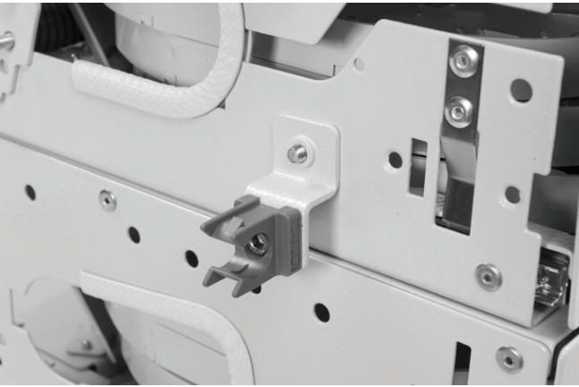
5.2.5 For 2HU only: install the flex tube holder on the bracket.
