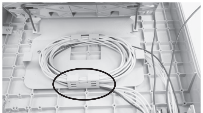
3.13 Use a wedge to support the trays. Store the loop on the looped bracket below the trays and secure the loop with two tie-wraps.
