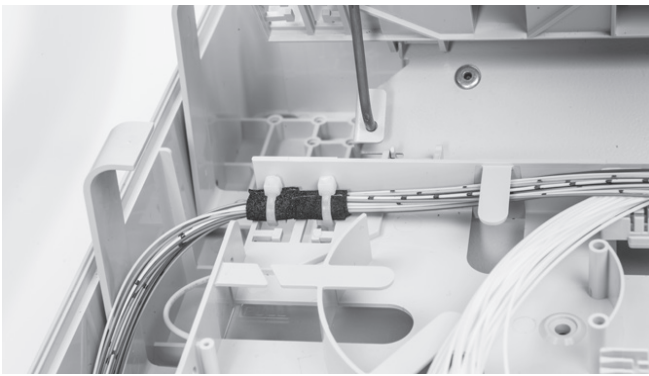
5.6 Secure the riser cable fibers into the tray with the foam and two tie-wraps.
