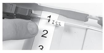
The identification (printed on the flags next to the connector boot) of the pre-assembled 900 micron pigtails is as follows
