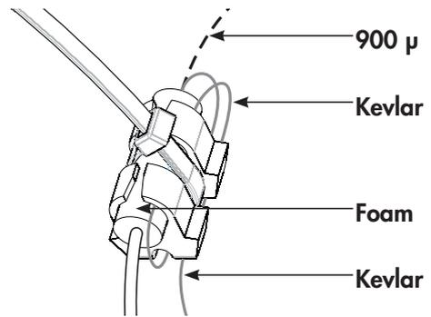
6.2 Wrap one layer of foam (20 mm) on the securing position if needed. Terminate the Kevlar by securing the cable/pigtail onto the bracket with tie-wrap. Depending the amount of Kevlar, it needs to be wrapped twice around the bracket.
