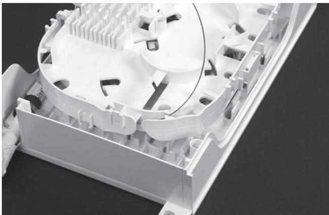
5.7 Fibers which will be spliced to the drop cables should be routed to the top side of the tray.
