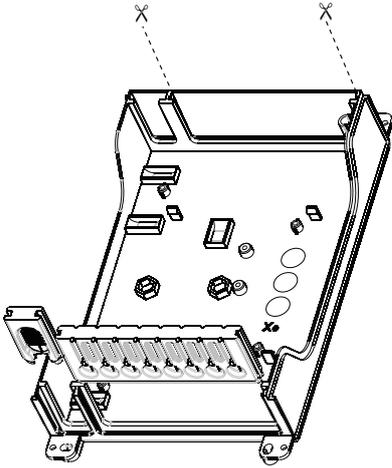
4.1 Break out the ports needed, For breaking out the ports, first cut with the scissor.
