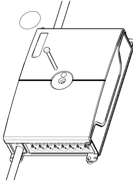
7.1 Secure the cover with the screw and seal with label (optional).
