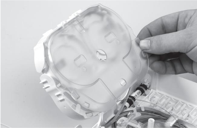
6.9 Install the covers (top/bottom) onto the tray.
