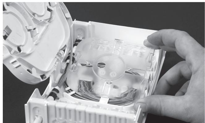
6.4 Install the cover on top of the stored uncut fibers.
