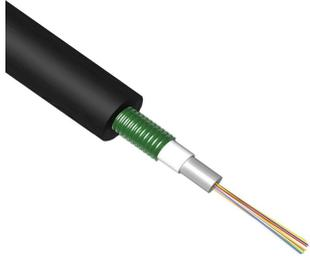
Fiber OSP cable, 12-fiber, OS2, HDPE, loose tube, 12 fiber, gel-filled, Singlemode G.652.D and G.657.A1, 1000 m, Meters jacket marking, Black jacket color. Provides Rodent Resistance.
