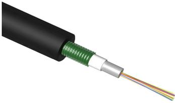
Fiber OSP cable, HDPE, 8-fiber, Singlemode, loose tube, gel-filled, Singlemode G.652.D and G.657.A1, Meters jacket marking, Black jacket color, 1000 m. Provides Rodent Resistance
