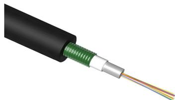
Fiber OSP cable, 12-fiber, OS2, HDPE, loose tube, 12 fiber, gel-filled, Singlemode G.652.D and G.657.A1, 1000 m, Meters jacket marking, Black jacket color
