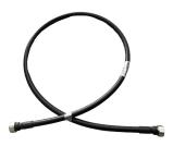
HELIAX® 1/2" Superflexible Fire retardant SureFlex® Jumper with interface types 4.3-10 Male and 7-16 DIN Male , 2m, with black non-halogenated fire retardant polyolefin jacket
