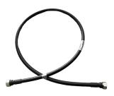
HELIAX® 1/2" Superflexible Fire retardant SureFlex® Jumper with interface types 4.3-10 Male and 7-16 DIN Male, 10 m, with black non-halogenated fire retardant polyolefin jacket
