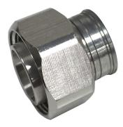
Product Classification **Product Type** Wireless and radiating connector **Product Brand HELIAX®** General Specifications **Body Style** Straight **Cable Family** RSJ4-50 **Inner Contact Attachment Method** Captivated Inner Contact Plating Silver Interface 7-16 DIN Male **Outer Contact Attachment Method** Solder **Outer Contact Plating** Trimetal Pressurizable No Dimensions Length 23.2 mm | 0.913 in Diameter 34.54 mm | 1.36 in **Nominal Size** 1/2 in
