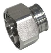
Product Classification **Product Type** Wireless and radiating connector **Product Brand HELIAX®** General Specifications **Body Style** Straight RSJ4-50 **Cable Family Inner Contact Attachment Method** Captivated Inner Contact Plating Silver Interface 4.3-10 Male **Outer Contact Attachment Method** Solder **Outer Contact Plating** Trimetal Dimensions Length 20 mm | 0.787 in Diameter 24 mm | 0.945 in **Nominal Size** 1/2 in
