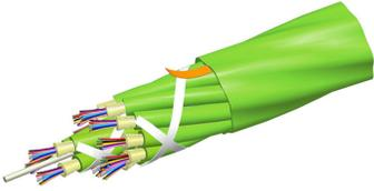
Fiber indoor cable, LazrSPEED® Plenum MPO Trunk, 144 fiber multi-unit with 16 fiber subunits, Multimode OM5, Gel-free, Feet jacket marking, Lime green jacket color
