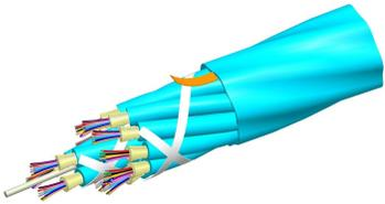
Fiber indoor cable, LazrSPEED® Plenum MPO Trunk, 288 fiber multi-unit with 12 fiber subunits, Multimode OM4, Gel-free, Feet jacket marking, Aqua jacket color
