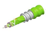
Fiber indoor cable, LazrSPEED Plenum MPO Trunk, interlocking aluminum armored with plenum jacket, 144 fiber multi-unit with 8 fiber subunits, Multimode OM5, Feet jacket marking, Yellow jacket color
