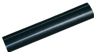
TCS2® Heat-Shrink Cable Seal, 48 inch long, 0.375 inch recovered ID, 0.08 inch recovered wall thickness
