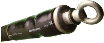
XCSM Thick-Wall Heat-Shrinkable Tubing kit, 85 mm/22 mm Shrink ratio, 1000 mm long, hotmelt adhesive, 5 pcs
