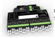
FACT® MPO Module, right sided, LC at front side, 2x12 fiber MPO at rear side, Ultra Low Loss (ULL) multimode OM5, wiring method A straight
