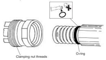
Add Clamping Nut and Cut Cable. Push the clamping nut fully onto the cable with a twisting motion so that the spring contacts snap into the second outer conductor corrugation valley and the O-ring seats properly against the inside surface of the clamping nut.
