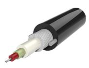
Fiber OSP cable, A2 Dual-sheathed HDPE Drop, LSZH Subunit, Loose buffer, Singlemode, G.657.A2, 1 fiber, Gel-free, Meters jacket marking, Black jacket color. (Cca class for subunit only)
