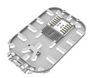
TENIO™ Rollable Ribbon Splice Tray for large closures (CH6 size) for up to 6 Ribbon splice protectors (72 Rollable ribbon fibers) + 12 single fiber heat shrink splice protectors (SMOUV 45 mm) per tray. Max capacity of 6 Rollable Ribbon trays per closure
