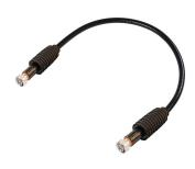
HELIAX® 1/2" SureFlex® Fire retardant Jumper with interface types 7-16 DIN Male and 7-16 DIN Male with HELIAX® SureGuard weatherproofing, with black non-halogenated fire retardant polyolefin jacket B2ca-S1a-d1-a1
