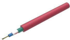
Fiber OSP cable, 6-fiber, HDPE, loose tube, gel-filled, Singlemode G.652. D and G.657.A1, Meters jacket marking, Red jacket color, 1000 m. Provides Rodent Resistance
