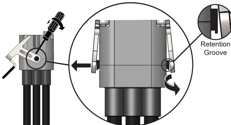
3 Once the latch is removed, bend the two arms back to 90° so they will fit tightly back onto the housing. To reattach, latch one arm over a hinge pin then roll other arm over the housing and onto the other hinge pin.
