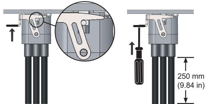
Keep 250 mm (9.84 in) length straight before routing to the device. First hanger should be located within 0.5 meter (19.6 inches).
