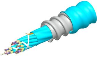
Fiber indoor cable, LazrSPEED® Riser/LSZH rated, MPO Trunk, interlocking aluminum armored, Multimode OM4, 144 fiber multi-unit with 12 fiber subunits, Gel-free, Feet jacket marking, Aqua jacket color
