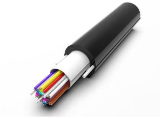
Fiber indoor/outdoor Retractable Façade Distribution Cable, 24 fibers, Singlemode, G.657.A1, Gel-free, Meters jacket marking, Black jacket color
