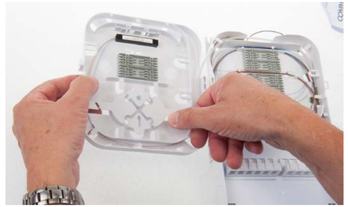
11.4 Put clear cover back. Splice feeder fiber, store splice protector and fiber over length properly.
