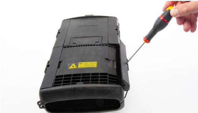
5.1 Open the closure by lifting the latches using a screw driver.
