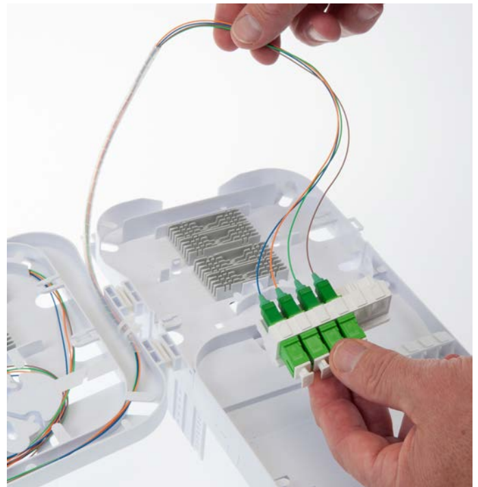
12.2 In order to route the midspan fibers underneath the transportation tube the adapter panel can be taken out easily.
