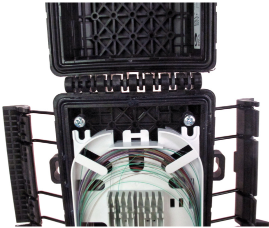
7.1 Install the organizer in the housing by sliding the organizer under the 2 screws.
