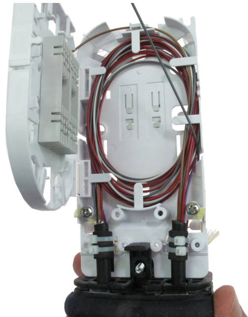
6.4.2 Route the bundle to the top of the tray. Use the slit for guiding the fiber bundle to the opposite side.
