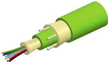
Fiber indoor cable, LazrSPEED® Low Smoke Zero Halogen Riser MPO Trunk with 2.0mm Subunits, 8 fiber, Multimode OM5, Gel-free, Meters jacket marking, Lime green jacket color, B2ca Flame rating
