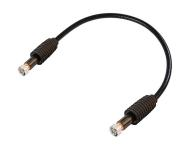
D-CLASS LDF4-50A SureFlex® Jumper with interface types 4.3-10 Male and 7-16 Din Male with HELIAX® SureGuard weatherproofing
