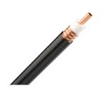
AVA5-50, HELIAX® Andrew Virtual Air™ Coaxial Cable, corrugated copper, 7/8 in, black PE jacket (Halogen free jacketing non-fire-retardant) tested C-Band and CBRS qualified.
