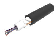
Fiber indoor/outdoor cable, 12-fiber, Singlemode G.652.D and G.657.A1, Gel-free, Meters jacket marking, Black jacket color, Dca flame rating, 2000 m. Provides Rodent Resistance
