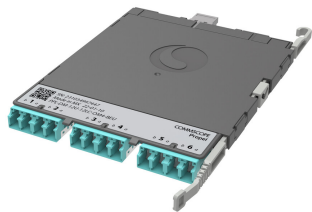
Propel ULL Multimode OM4 MPO-12 Distribution Module, 6 duplex LC to 1X12f MPO/UPC non-pinned, Method B Enhanced
