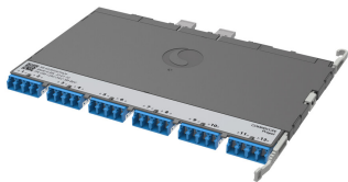
Propel ULL Singlemode MPO-12 Distribution Module, 12 duplex LC/UPC to 2X12f MPO/APC non-pinned, Method B Enhanced
