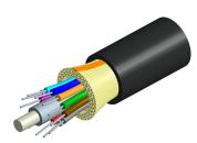
Fiber Indoor/Outdoor cable, LazrSPEED®, Low Smoke Zero Halogen Riser Distribution Cable, 24 fiber single-unit, Gel-free, Multimode OM3, Feet jacket marking, Black jacket color, Dca flame rating
